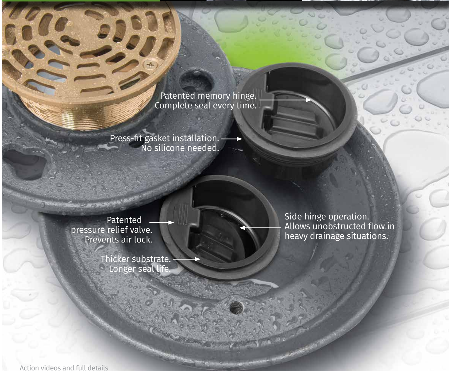
SureSeal press-fit installation
