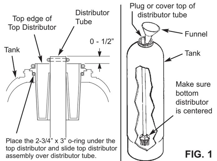
Place the 2-3/4" x 3" o-ring under the top distributor and slide top distributor assembly over distributor tube.
