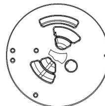
Rotor & Disc, Multiple Tank, Filters & Softener Model 071
