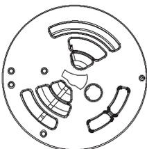
Rotor & Disc, Single Tank, Filters & Softener Model 071
