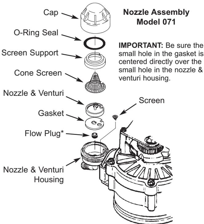
\*Install with numbered side up, concave side down.
