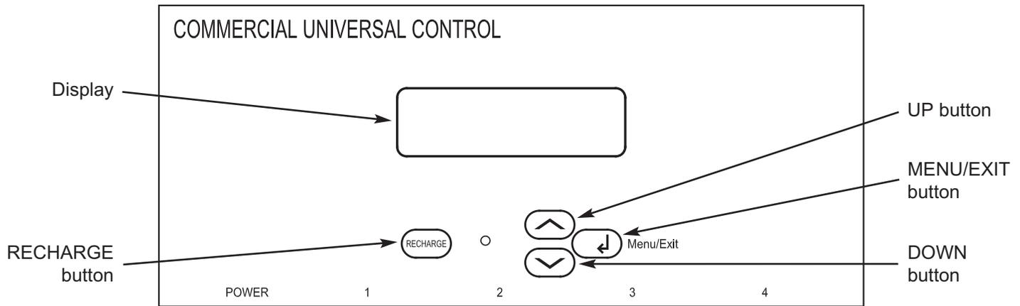
The CUC2 is a menu-driven electronic controller with a dot matrix display. The UP ( $\blacktriangle$ ) and DOWN ( $\blacktriangledown$ ) buttons move the cursor ( $\>$ ) up and down the menu choices. The MENU/EXIT ( $\leftarrow$ ) button enters the value selected and returns the display back a level. The controller will return to the normal operating screen after 4 minutes, if left in a menu and no selection has been made.
